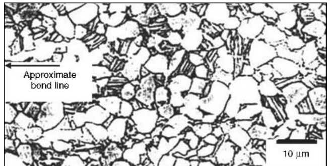
Fig. 8 Metallography of bond quality produced using the stop-off process
